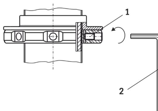
Fix the spring plate with the set screw (1) by using hex key (2) delivered by BILSTEIN.
