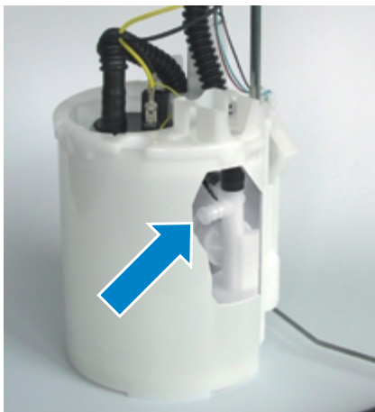
Fig. 1: View into the fuel delivery module (elevation) with blind-mate connector
