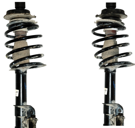
Correctly fitted top plate
