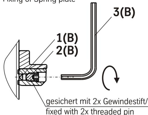
Fix the spring plate with the rubber pins/balls (1) and set screw (2) by using the auxiliary tool (hex key (3)).
