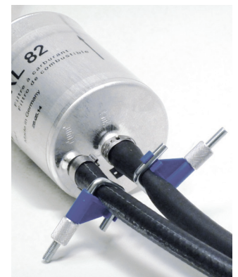
Figure 3: Pinching off the lines prevents air from penetrating into the fuel system.
