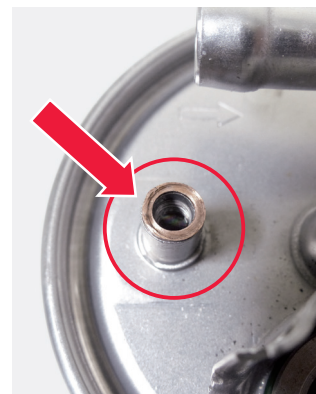
Figure 2: Sealing of the drain screw on the diesel fuel filter KL 154.
