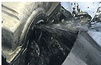
Attention: When the lubricating supply is working properly, the flow here can be 30–60 litres an hour.
