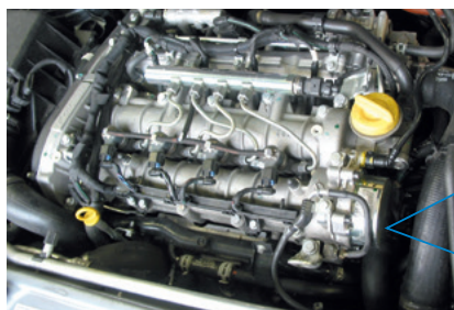
Example: On the Opel Vectra the lubricating oil feed is via bores in the flange
