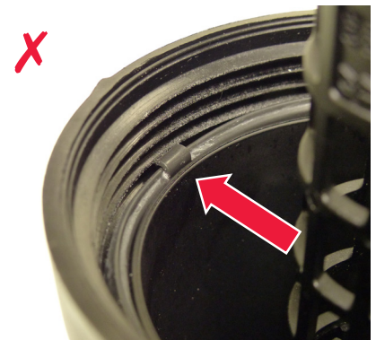
Figure 4: Spring fixing plate stuck in the thread
