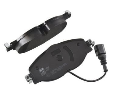
benefits and features - such as chamfering and/or the addition of slots to 'tune' the pad so it makes less noise. The chamfers and slots change the natural frequency at which the brake pad oscillates so it runs quieter than a brake pad without these features.
