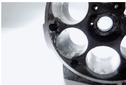
Figure 1: Piston seizure on the air conditioning compressor due to too much contrast agent
