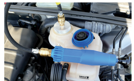
Figure 2: Pressure can also be applied to test the valve in the cap by using special adapters.
