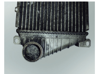
Figure 2: Chips from the destroyed impeller in the charge air cooler
