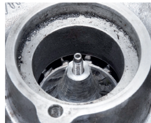
Figure 1: Impeller completely destroyed by foreign objects
