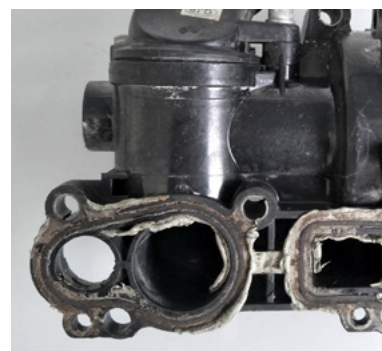
Fig. 5: Leakage due to additional sealant (damage symptoms)
