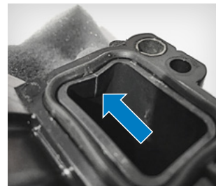
Fig. 2: Breakage (damage pattern)
