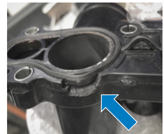
Fig. 3: Breakage (damage pattern)
