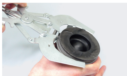
Figure 2: Fit the rings using suitable piston ring pliers.
